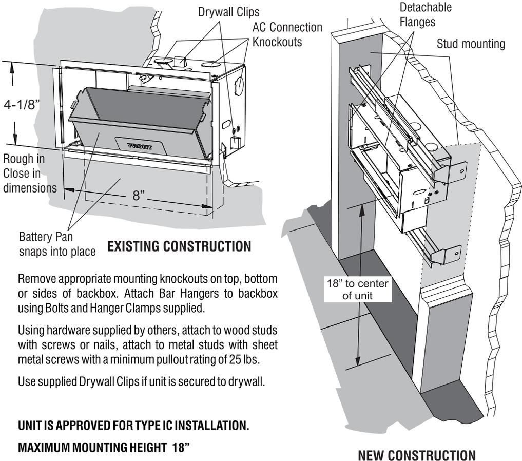
Remove appropriate mounting knockouts on top, bottom or sides of backbox. Attach Bar Hangers to backbox using Bolts and Hanger Clamps supplied.
