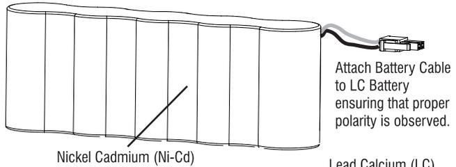
Attach Battery Cable to LC Battery ensuring that proper polarity is observed.
